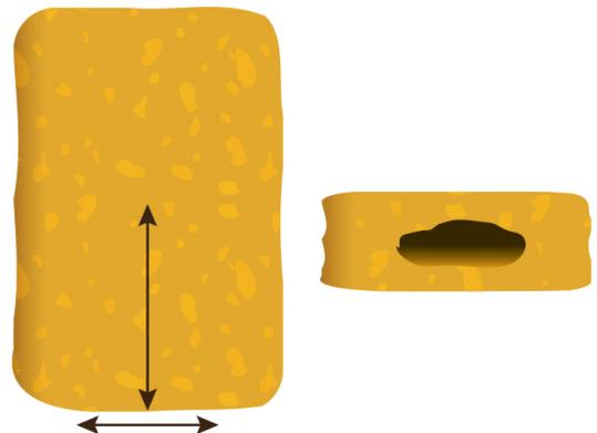
3. Insert the leashed temperature sensor. Remove additional sponge material if needed to make sure the sensor stays firmly in place.
