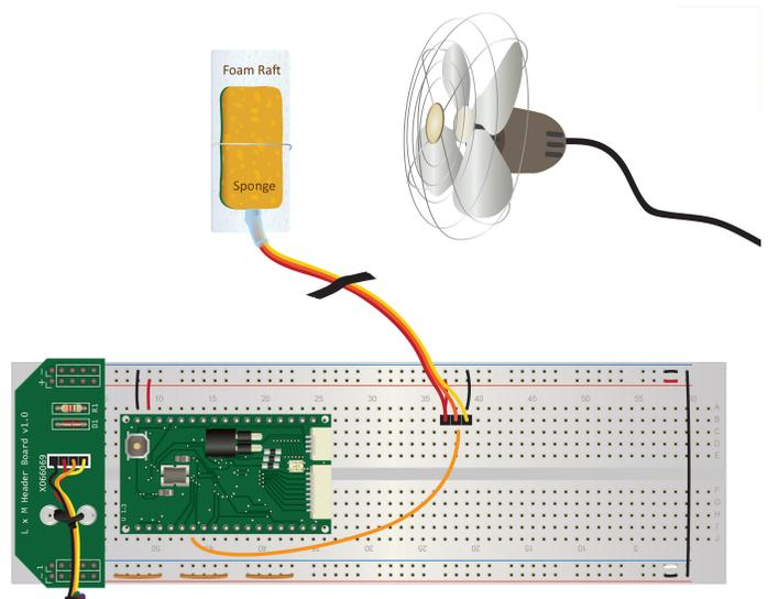
2. Create a cavity inside the sponge for the sensor. Use scissors to cut out a hole large enough to place the temperature sensor in the middle of the sponge.
